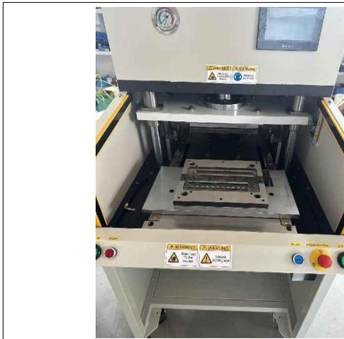
Picture 7 Hazard 1.2, Image 1, Loading opening and warning signs
