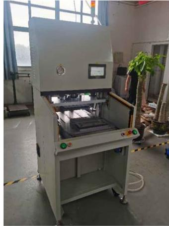
Picture 1 15T FPC Punch Machine general view
