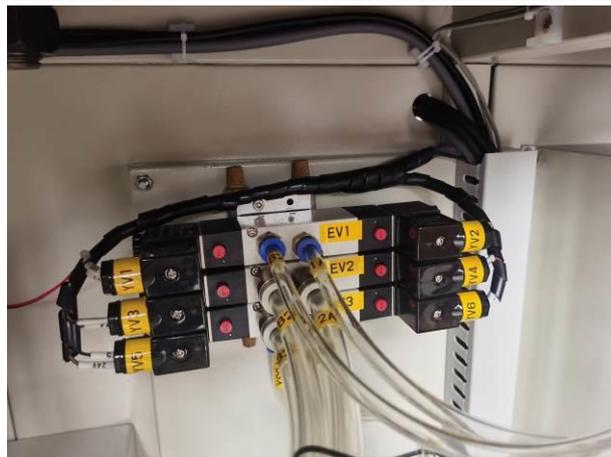
Picture 18 Hazard 3.2, Image 1, 5/3-way with mid-position exhausted
