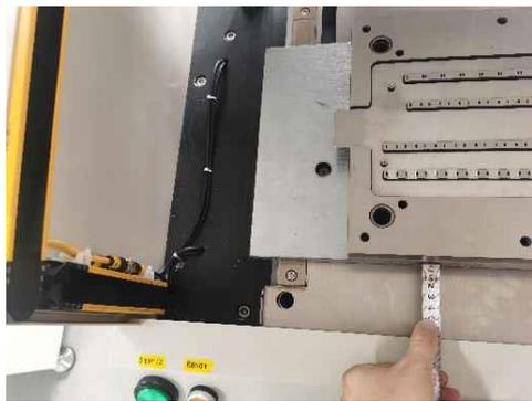
Picture 9 Hazard 1.2, Image 3, Safety distance is about 50mm
