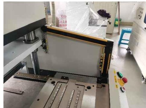
Picture 5 Hazard 1.1, Image 2, Loading opening
